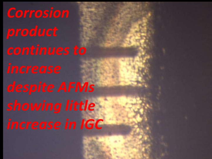
*TL-AFMs at (a) 30, (b) 60, (c) 120, (d) 240 minutes Immersion at open circuit potential in 1 Mol dm<sup>-3</sup>*
